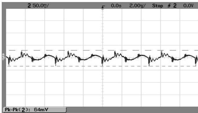
Transient Response (Vin=48V, Iout=50-75-50% of Imax) (Recovery time=9.6uS)
