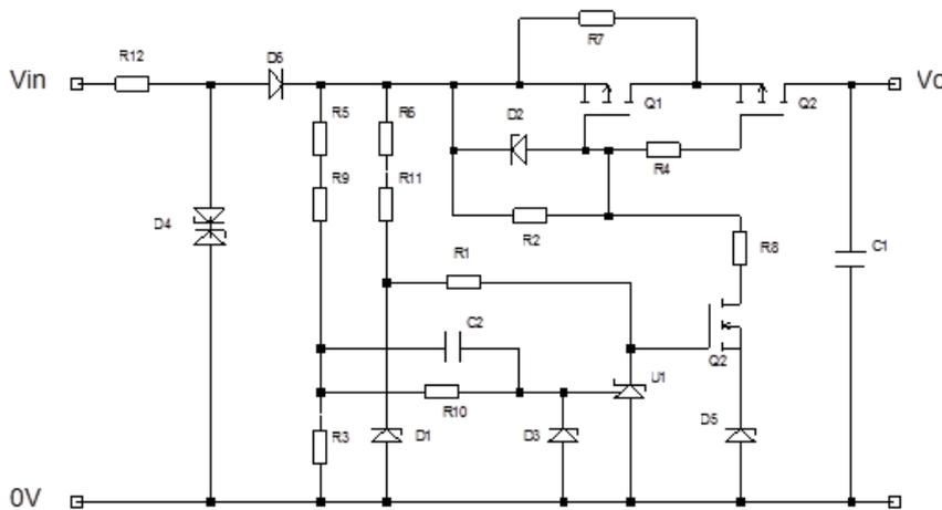
This circuit has been evaluated successfully over temperature for nominal 110 VDC input worst case 3.5 Vnom surge as specified in RIA12. Waveforms obtained are shown in Figures 3. Suggested component values for 110V input are given in Table 4.
