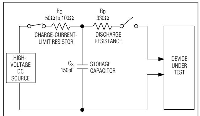
Figure 8. IEC 61000-4-2 ESD Test Model
