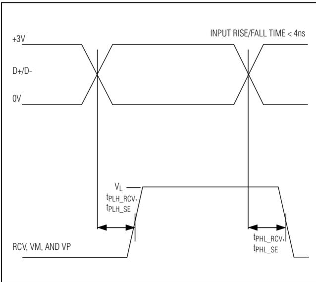
Figure 4. D+/D- Timing to VP, VM, and RCV
