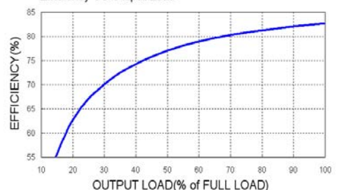
DUR01-24S12 Efficiency VS Output Load
