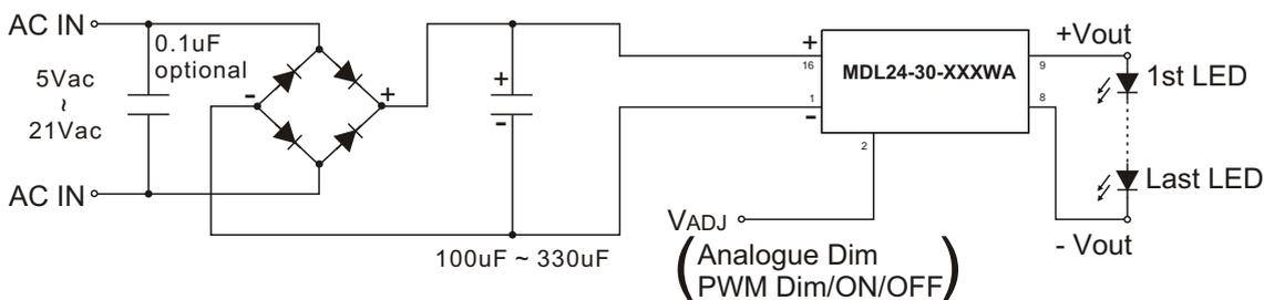
Output Current Adjustment By External DC Control Voltage
