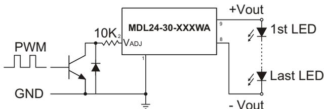
**Driving the ADJ input from a microcontroller**
