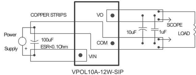
Figure 16. Output Voltage Ripple and Noise Measurement Set-Up
