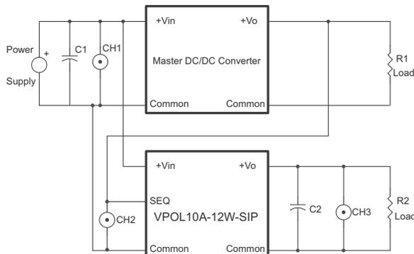
Figure 5. Example testing circuit of sequencing function
