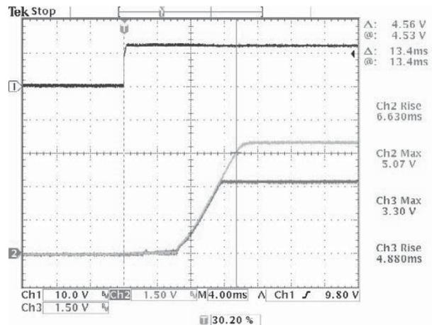
Figure 6. Example testing circuit of sequencing function
