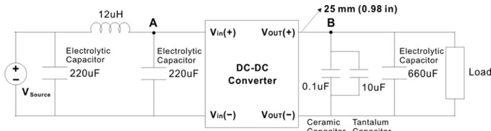
1. During the test of input reflected ripple current, the input terminal must be connected to a 12 uH inductor and a 220 uF electrolytic capacitor.
