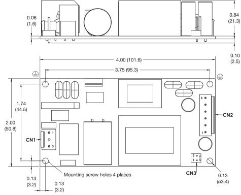
Mounting holes marked with (a) must be connected to safety earth
