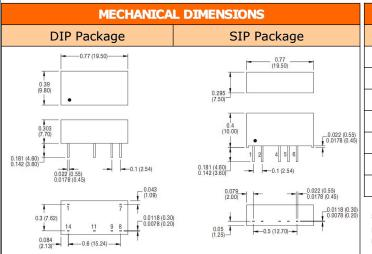
All dimensions in inches  $\pm 0.01(mm\pm 0.25mm)$ . All pins on a 0.1(2.54) pitch and within  $\pm 0.01(0.25)$  of true position. Weight: 2.4g (DIP) 2.1g (SIP)
